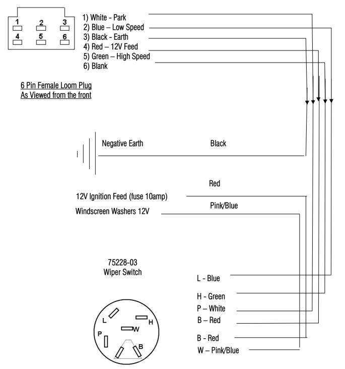
Wiper switch system is 12V Positive Feed
